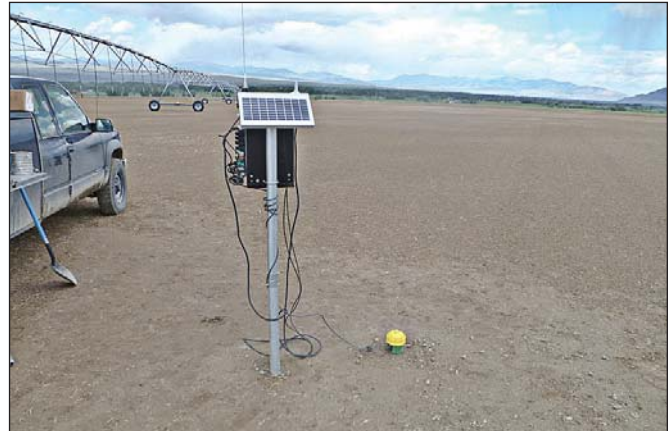
A soil moisture monitoring station near Silver Star.
