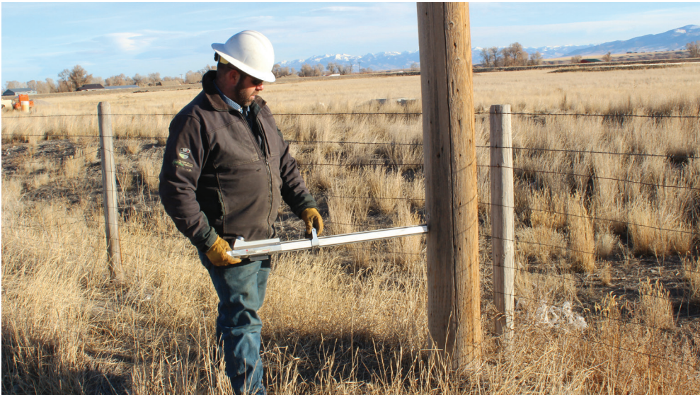
Lineman Cody Tarter demonstrates a pole-testing drill. | VIGILANTE FILE PHOTO
